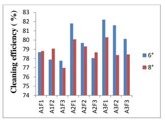
Fig. 4. Effect of screen slope on cleaning efficiency (%) for flat screen grain pre- cleaner.
