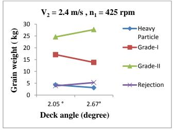
Fig. 13. Effect of deck angle on grading quality of grain for gravity separator.
