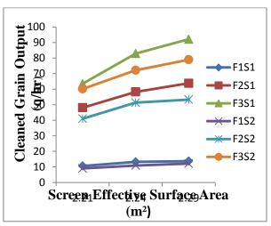
Fig. 7. Effect of screen effective surface area on cleaned grain output as affected by feed rate, screen slope and air velocity for flat screen grain pre-cleaner.
