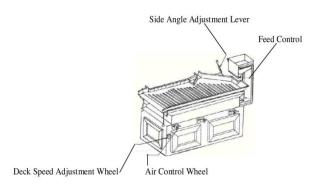
Fig. 2. Specific Gravity Separator
