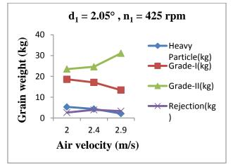
Fig. 11. Effect of Air velocity on grading quality of grain for gravity separator.
