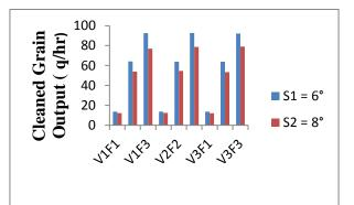
Fig. 8. Effect of screen slope on cleaned grain output for flat screen grain pre- cleaner.
