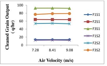
Fig. 9. Effect of air velocity on cleaned grain output as affected by different feed rate, screen slope and screen effective surface area for flat screen grain pre-cleaner.
