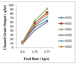
Fig. 10. Effect of feed rate on cleaned grain output as affected by different screen effective surface area, screen slope and air velocity for flat screen grain pre- cleaner.
