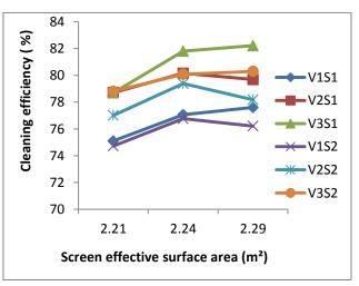
Fig. 3. Effect of screen effective surface area on cleaning efficiency as affected by air velocity, screen slope and feed rate for flat screen grain pre-cleaner.
