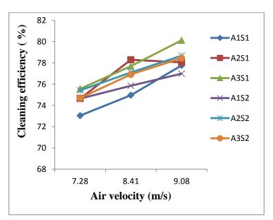
Fig. 5. Effect of air velocity on cleaning efficiency as affected by screen effective surface area, screen slope and feed rate for flat screen grain pre cleaner.
